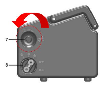
Purge your external tubes. For that put the inlet valve in the position shown with an arrow during 10s.
