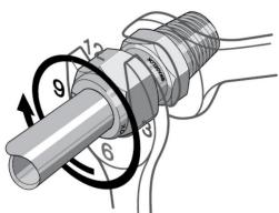
If the screw thread is damaged, the tightness of the screw thread will be not efficient and the oxygen measurement will be not reliable.
