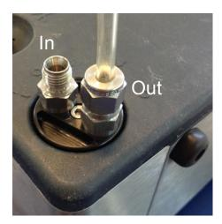
When you screw the tubing on the instrument, take care to use 2 flat leaf screws as mentioned in the following picture in order to not damage the screw threads of the plastic parts where the swagelok is screwed.
