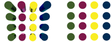
Left: non-telecentric optics Right: telecentric optics
