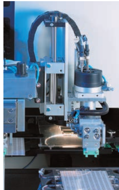
Laser trimming of platinum-chip temperature sensors
