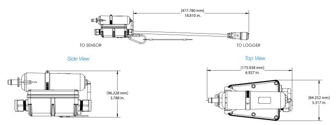
Desiccant Hub Assemblies for use with portable FL900 Series Loggers. (Sensor cable for use with FL1500 will not contain a desiccant hub and will have bare wires on cable end. Order Prod. No. 8321200 for desiccant cartridge to attach to FL1500.)
