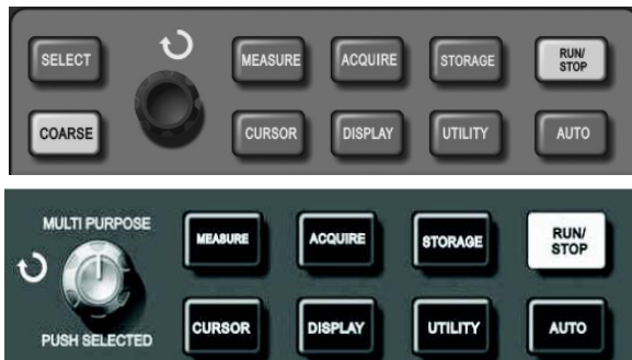
Figure 2 – 22 Function key (storage) for sampling system STORAGE key can be used to display storage setup menu. You can save oscillograph waveform or setup status to internal storage area or U disk to call out saved waveform by RefA (or RefB) or call out setup status by STORAGE key. Waveform display area of oscillograph can be saved to DSO contents in U disk in a form of bitmap. Saved bitmap can be read by PC computer.
