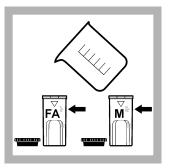
2. Fill two sample cells to the 10-mL line with sample. Write **FA** (free ammonia) on one sample cell. Write **M** (monochloramine) on the second sample cell.
