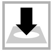
22. Insert the free ammonia sample cell into the cell holder. Point the diamond mark on the sample cell toward the keypad.
