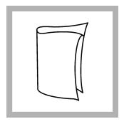
21. Clean the free ammonia sample cell. Make sure that there are no air bubbles in the sample cell after the reaction. If there are bubbles, invert the sample cell to remove the bubbles.
