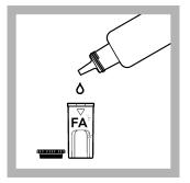
8. Add 1 drop of Free Ammonia Chlorinating Solution to the free ammonia sample cell. Close the reagent bottle to keep the reagent stable.
