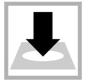
**4.** Insert the **monochloramine** sample cell into the cell holder. Point the diamond mark on the sample cell toward the keypad.
