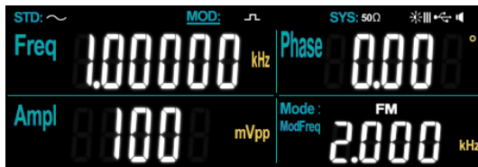
Picture 4-12 Set FM modulation frequency and waveform
