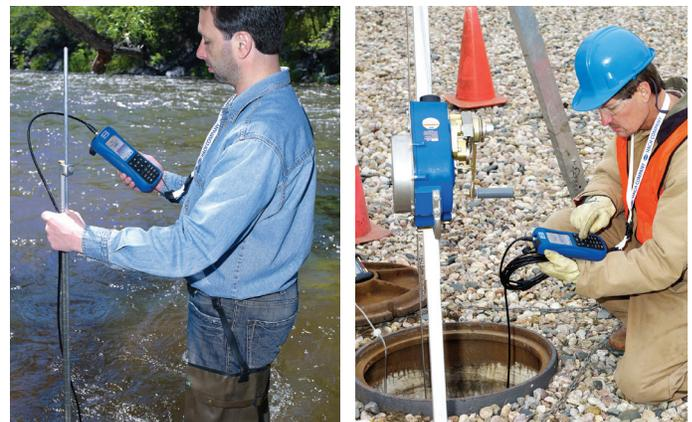
*Quickly profile streams and rivers. Easily verify other metering tools or use to select optimal monitoring sites.*
