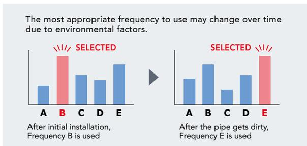
Unlike conventional flow meters, which typically use only one frequency for their ultrasonic signal, the FD-R Series continuously tests various frequencies to determine the ideal fit in every situation. By selecting the signal that travels through the pipe, liquid, and potential build-up with the least amount of loss, the FD-R Series is able to ensure proper flow monitoring.
