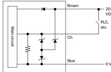
**(3) Wiring of channel to which analog output has been selected**
