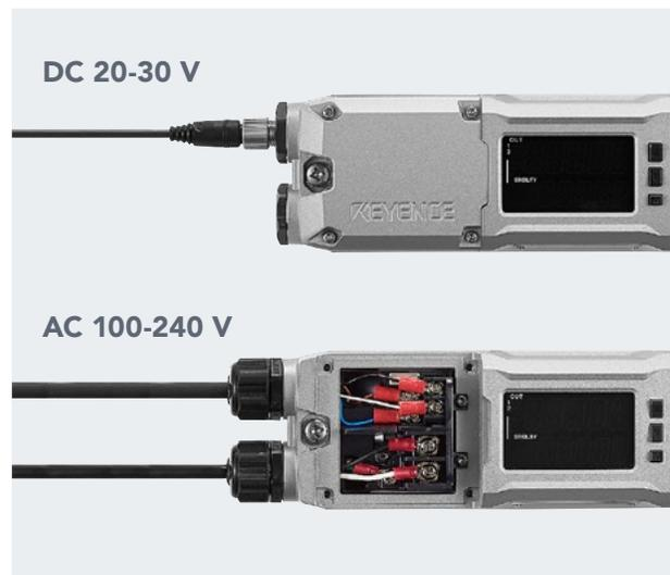
Perfectly integrate into any system with the ability to operate using either AC or DC power supplies.
