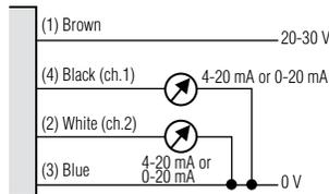
When you select ch.1: Analog, ch.2: OFF, independently insulate the white wire (2).
