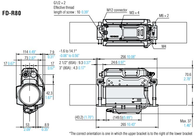
\*The correct orientation is one in which the upper bracket is to the right of the lower bracket
