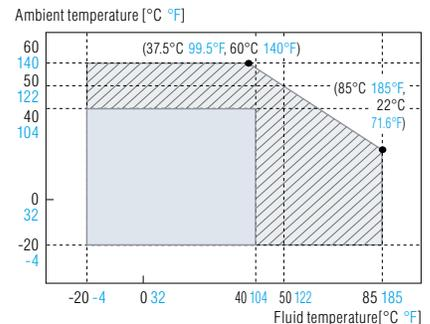
When using the FD-R Series in the temperature condition shown by oblique lines, use cables with heat resistance of 90°C 194°F or higher for the power cables and the I/O cables.
