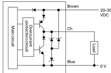
**(2) Wiring of channel to which external input has been selected**
