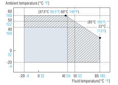
When using the FD-R Series in the temperature condition shown by oblique lines, use cables with heat resistance of 90°C 194°F or higher for the power cables and the I/O cables.
