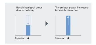
The stable transmission of the ultrasonic signal is imperative for consistently stable detection. Build up or rust on the inside of a pipe can become problematic over time for conventional flow sensors. By utilizing the Automatic Build-Up Resistance Function, the FD-R automatically adjusts its power to compensate for this build-up and provide lasting stable detection.
