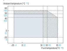
Temperature range when supplying AC power to the unit and being exposed to radiation such as direct sunlight.
