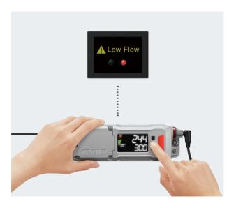
Conveniently check that the outputs are connected properly without needing to change the actual flow rate or temperature.
