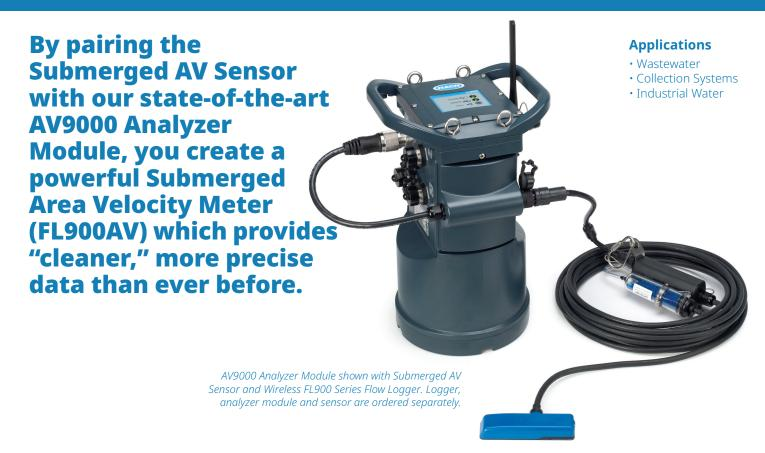
Our **Submerged AV Sensor** is a robust, 1 MHz Acoustic Doppler velocity sensor designed to measure wastewater flow with improved accuracy and reliability. This tried-and-true sensor also uses a pressure transducer to measure flow level and incorporates advanced technologies to ensure precision, including automatically correcting for temperature and velocity effects on measurements.
