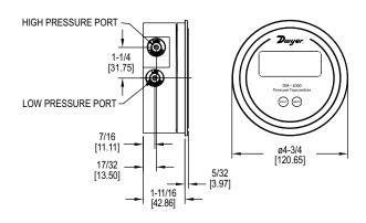
The Dwyer Series DM-2000 Differential Pressure Transmitters sense the pressure of air and compatible gases and sends a standard 4-20 mA output signal. The DM-2000 housing is specifically designed to mount in the same diameter cutout as a standard Magnehelic® gage. A wide range of models are available factory calibrated
