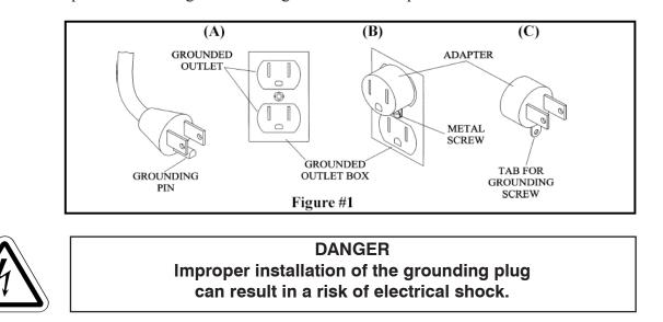
If repair or replacement of the cord or plug is necessary, do not connect the grounding wire to either flat blade terminal. The wire with insulation having an outer surface that is green with or without yellow stripes is the grounding wire.
