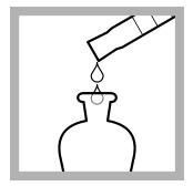
**9.** Add 20 mL of 50% Sodium Hydroxide Solution to the funnel.
