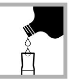
6. Prepare the DithiVer solution: Add 30 mL of chloroform to a 50-mL mixing cylinder.
