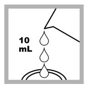
**20. Prepare the blank:** Put at least 10 mL of chloroform in a dry sample cell. Put the stopper on the sample cell.
