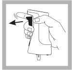
1. If the blue indicator button doesn't retract when the trigger is released, hold the dispenser with the dispensing tip up and engage the trigger fully.
