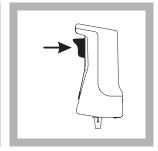
**4.** To dispense the powdered reagent, invert and grip so that the index finger is over the trigger. Engage the trigger fully, then release it quickly.
