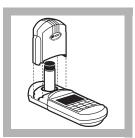
**14.** Immediately place the prepared sample into the cell holder. Tightly cover the sample cell with the instrument cap.
