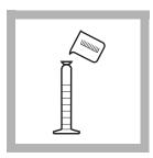
**3.** Fill a 50-mL graduated mixing cylinder to the 50-mL mark with sample.
