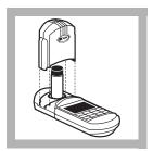
12. Within three minutes after the timer beeps, place the blank into the cell holder. Tightly cover the sample cell with the instrument cap.
