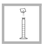
**8.** Add the contents of one Bleaching 3 Reagent Powder Pillow to the remaining 25 mL in the mixing graduated cylinder (the blank). Stopper the cylinder.
