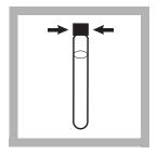
**5.** Replace the vial cap tightly. Rinse the outside of the COD vial with deionized water and wipe the vial clean with a paper towel.
