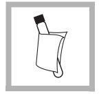
**4.** Clean the outside of the blank with a towel. *Note:* Wiping with a damp towel, followed by a dry one, will remove fingerprints or other marks.
