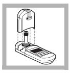
**10.** Tightly cover the vial with the instrument cap.
