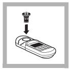
**3.** Insert the COD/TNT Adapter into the cell holder by rotating the adapter until it drops into place. Then push down to fully insert it.
