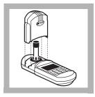
**6.** Tightly cover the sample cell with the instrument cap.
