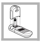
**6.** Tightly cover the vial with the instrument cap. Note: The blank is stable when stored in the dark. See Blanks for Colorimetric Determination following these procedures.
