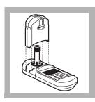
**10.** Tightly cover the sample cell with the instrument cap.
